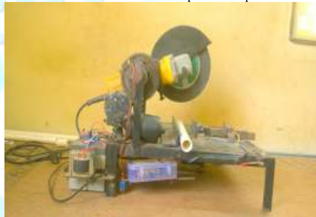
Figure 1 SET UP OF PIPE CUTTING USING RACK AND PINION MECHANISM
